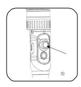
⑤ Mode switch You can switch to different working mode by pressing the 5-way joystick. Please refer to the following introduction.
