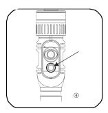
④ Power on Power on the Gimbal. Press the function button until the indicator flashing twice.
